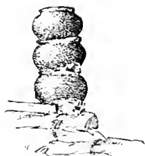
POT CHIMNEY. AS BUILT BY INDIANS IN THE N.W. OF THE U.S.
